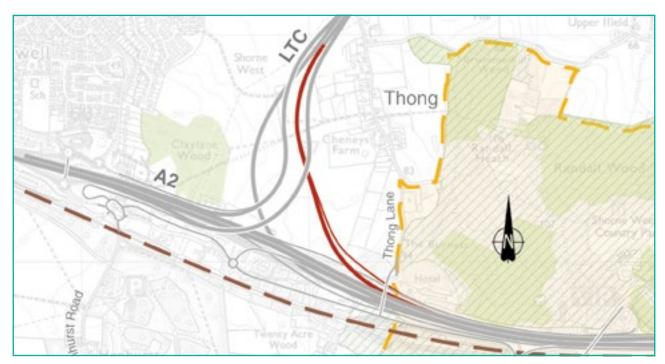
Figure 5-1. **Leaving the LTC to join the M2/A2 eastbound.** Slip road leaving the LTC southbound divides to connect to both the M2/A2 and the eastbound parallel link road (which leads to local roads). The road passes under the LTC in a cutting before being elevated on an embankment and passing over the A2 eastbound parallel link road
