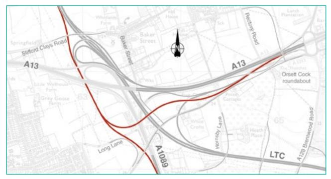
Figure 5-27. **Joining the LTC northbound from the A13. Traffic leaving the A1089 northbound also joins this connection.** This connection is in a cutting as it leaves the A13 at Orsett Cock. It travels under the realigned Orsett Cock roundabout A13 westbound on slip road, over the A13 westbound to the LTC southbound and the A1089. It is in a cutting to pass under the A13 and Stifford Clays Road and joins the LTC northbound
