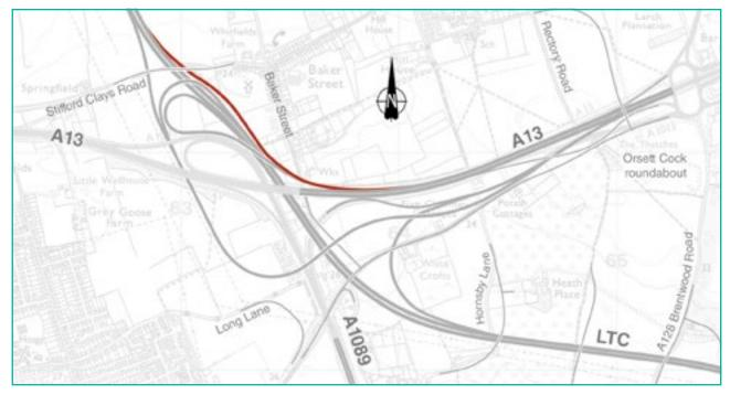
Figure 5-26. LTC southbound to join the A13 eastbound, joins with the connection from LTC northbound (figure 5-25). This connection will start in a cutting to pass under Stifford Clays Road before merging with the connection from the LTC northbound, passing over Baker Street and joining the A13
