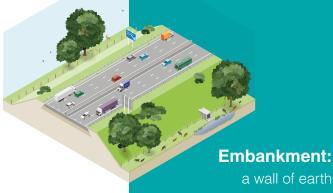
a wall of earth or stones to support a road, or to stop water from flooding an area.
