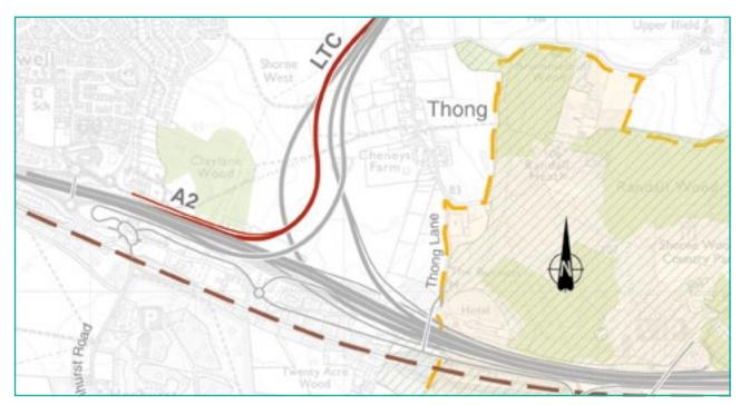
Figure 5-3. **Joining the LTC from the A2 eastbound and slip road from the Gravesend east junction.** The connection will be elevated on an embankment and will pass over the M2/A2 westbound to the LTC northbound twice to merge on the left
