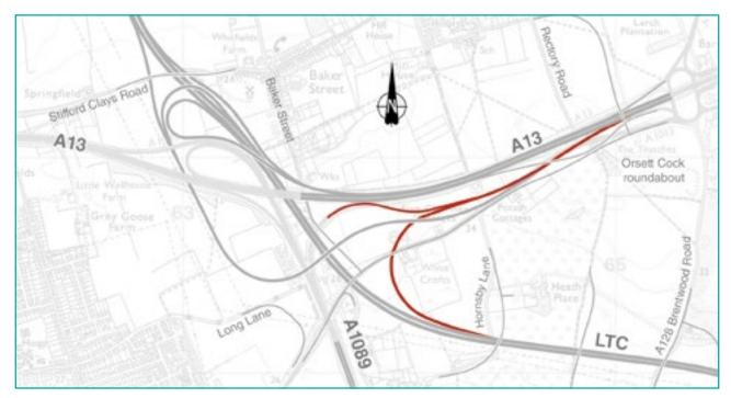
Figure 5-28. Leaving the A13 westbound to join the LTC southbound joins a connection to A1089 southbound (this will require changes to the existing A13 westbound to A1089 southbound slip road). This connection leaves the A13 westbound in a cutting under the realigned Orsett Cock roundabout A13 westbound on slip road. It is also in a cutting beneath the A13 to the LTC northbound and the A1013 before joining the LTC
