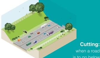
when a road is to go below existing ground, the soil or rock is removed, either altogether or to form landscape embankments on each side.
