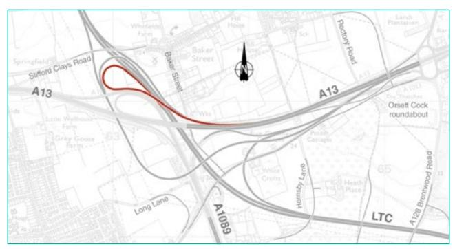
Figure 5-25. **LTC northbound to join the A13 eastbound.** This connection will start in a cutting before rising to cross the LTC and merge with the connection from the LTC southbound on an embankment, passing over Baker Street and joining the A13
