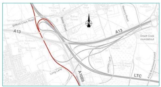
Figure 5-29. Leaving the A1089 northbound to join the LTC northbound and southbound. This connection leaves the A1089 in cutting under the A1013, remaining in a cutting to pass under the A13 and Stifford Clays Road, then joins with the LTC northbound. The LTC southbound connection diverges after passing under the A13 and crosses over the LTC to merge on the left.
