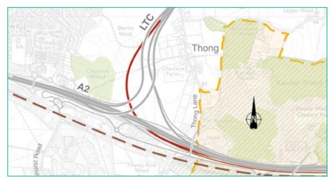
Figure 5-4. **Joining the LTC from the M2/A2 westbound.** Traffic from the westbound parallel link road will also join here. The road will be in a cutting, passing below the A2 main road and two LTC slip roads
