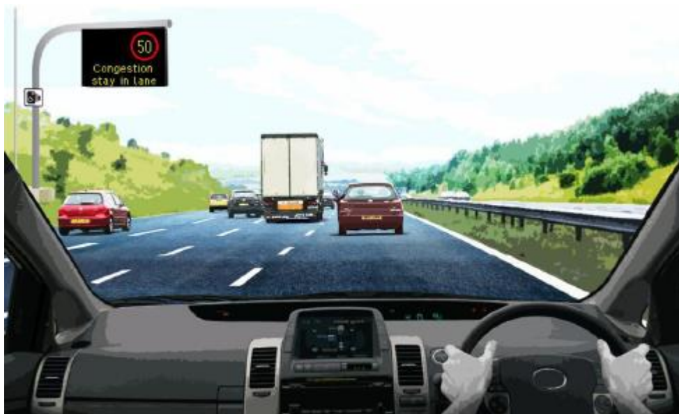
Figure 4d: Illustrative smart motorway scheme section operating with variable mandatory speed limits and information for road users
