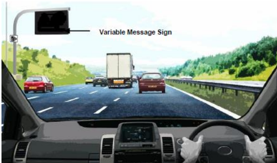
Figure 4b: Illustrative smart motorway all-lane running scheme section operating in normal motorway conditions with a blank cantilever mounted variable message sign
