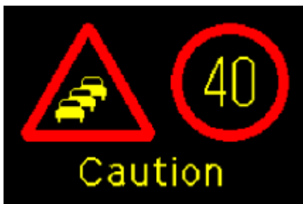
Figure 4f: Variable message sign with a warning pictogram displaying queue caution information and a reduced mandatory speed limit
