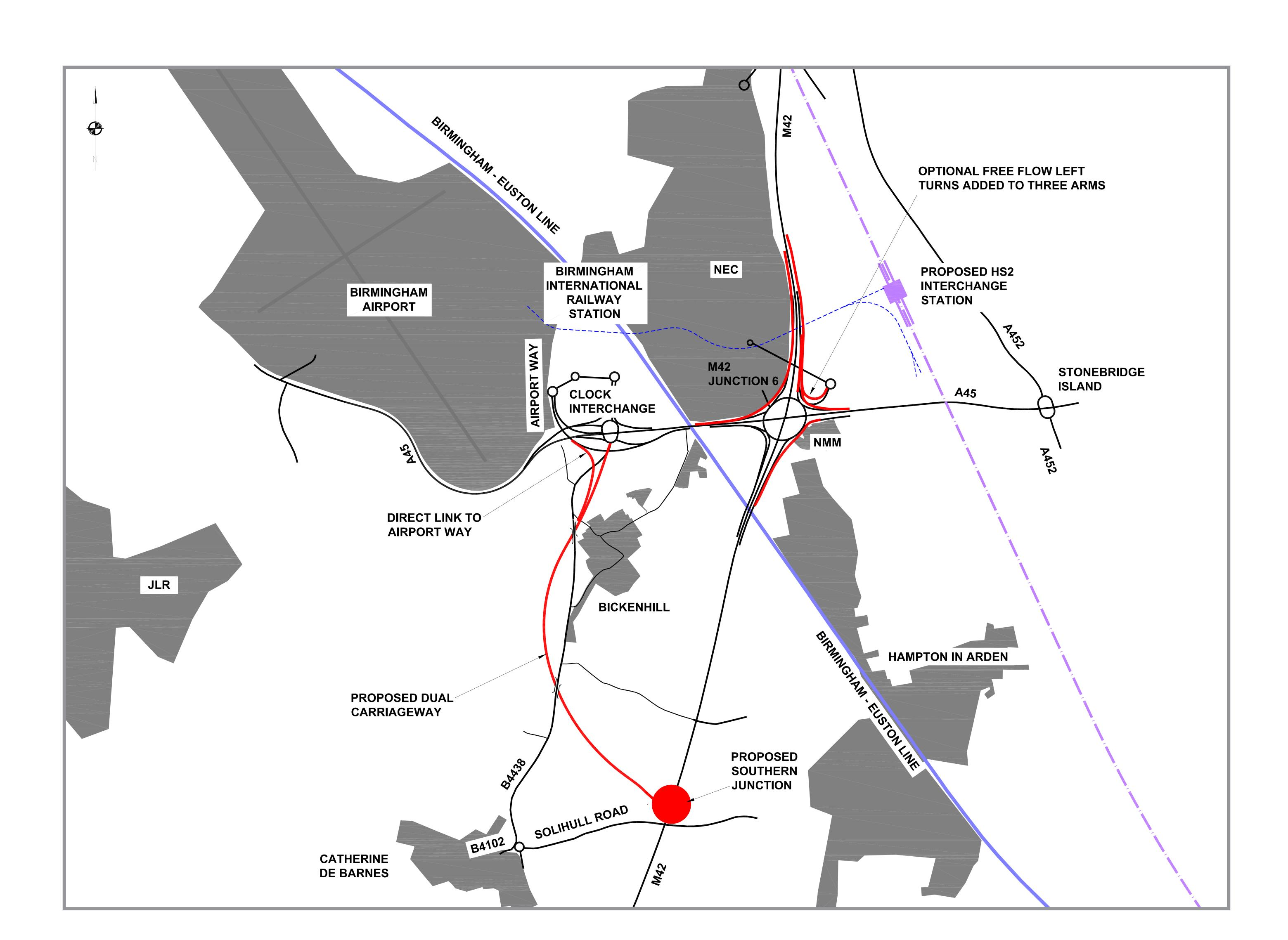
This option would provide a new 2.4 kilometre dual carriageway link between the Clock Interchange and an all movements junction allowing north and south access to the M42 north of Solihull Road. The Clock Interchange would be improved to accommodate the additional flows and a free flow link would be provided to give improved access to Birmingham Airport and A45 west.
