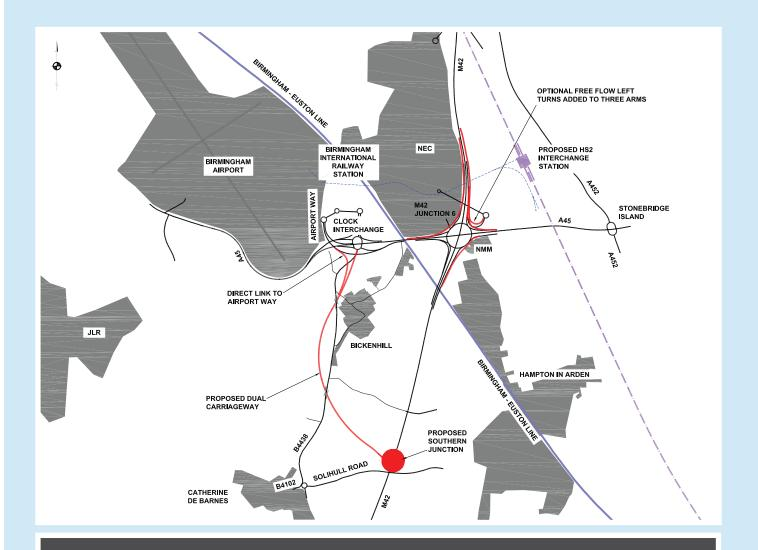
This option would provide a new 2.4 kilometre dual carriageway link between the Clock Interchange and an all movements junction allowing north and south access to the M42 north of Solihull Road. The Clock Interchange would be improved to accommodate the additional flows of traffic, and free flow links would be provided to give improved access to Birmingham Airport and A45 west.
