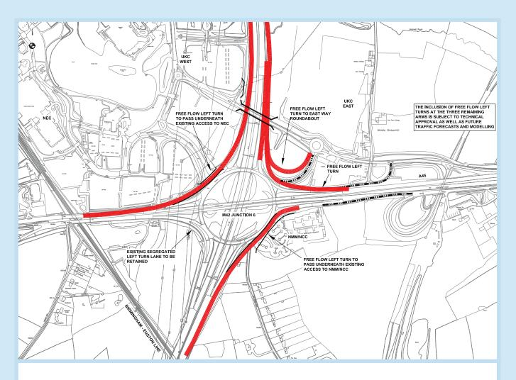
Whichever option we take forward, there is the potential to maximise the improvement at M42 junction 6 even further by providing dedicated free flow left turns.
