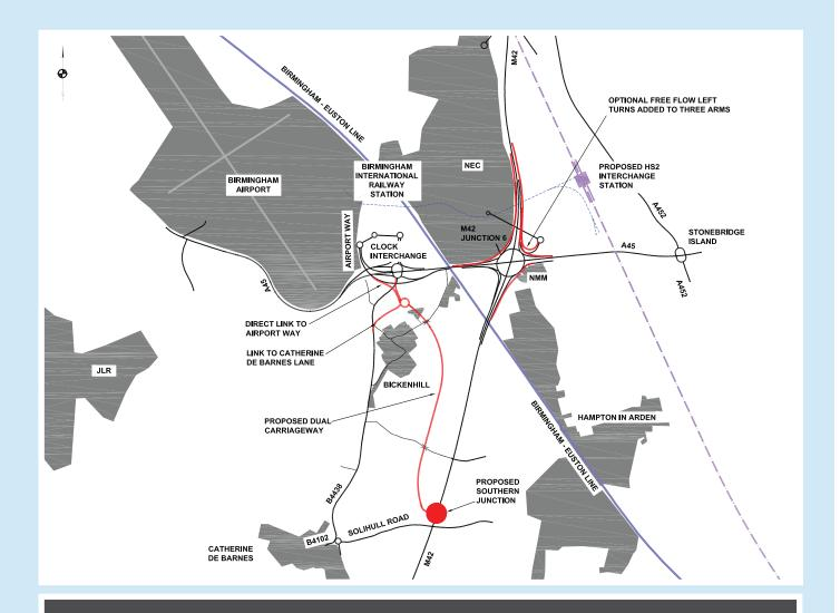
This option would provide a new 2.3 kilometre dual carriageway link between the Clock Interchange and an all movements junction allowing north and south access to the M42 north of Solihull Road. The Clock Interchange would be improved to accommodate the additional flows of traffic and a free flow link would be provided to improve access to Birmingham Airport and A45 west.
