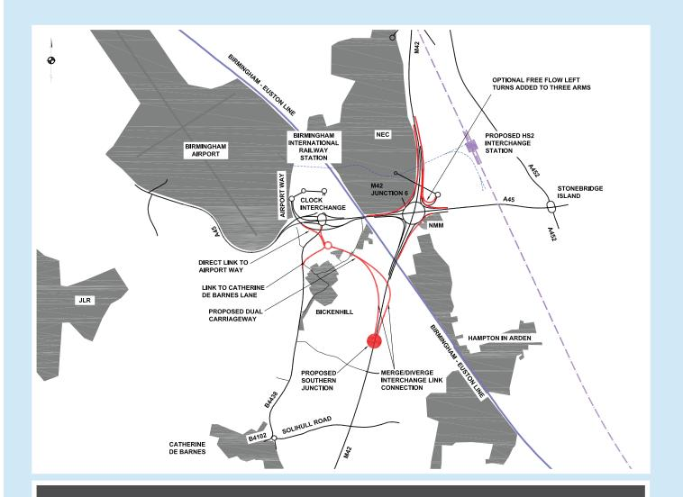
This option would provide a new 1.6 kilometre dual carriageway link between the Clock Interchange and a restricted movements junction with the M42 north of Shadowbrook Lane. This junction would only enable traffic to join the M42 southbound or exit the M42 northbound using free flow links. The Clock Interchange would be improved to accommodate the additional flows of traffic and a free flow link would be provided to improve access to Birmingham Airport and A45 west.
