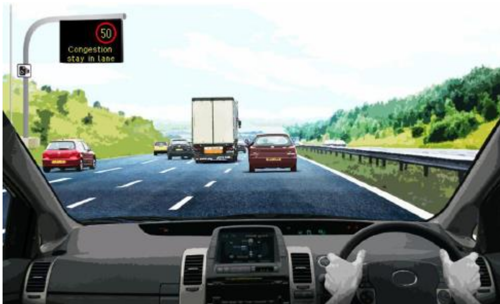
Figure 4d: Illustrative smart motorway all-lane running scheme section operating with variable mandatory speed limits and information for road users
