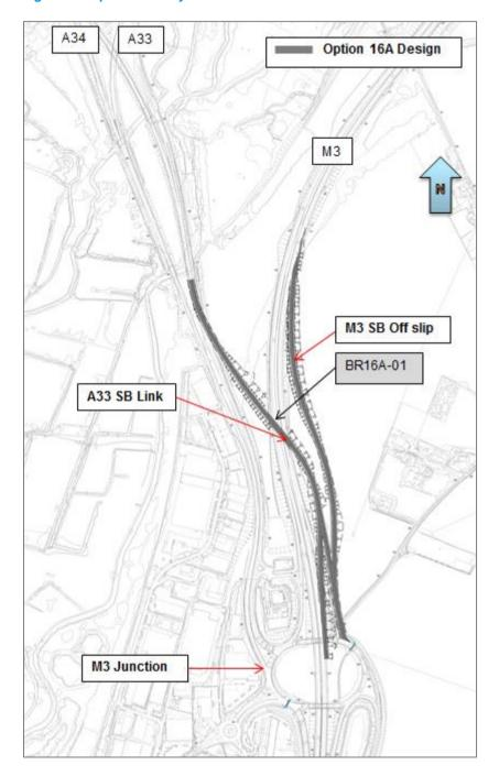
5.10.2 Option 16A proposes the incremental delivery of only the A34 southbound link associated with Option 14. This option has been developed as a potential means of partially meeting the scheme free flow objective at a more affordable cost. Option 16A could be combined with 16B at a later stage to effectively provide Option 14 in two phases/schemes, however this is expected to be more expensive in the long term than building Option 14 initially.
