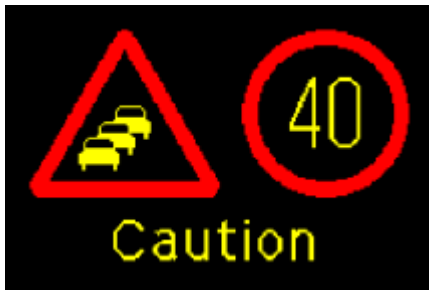
Figure 4f: Variable message sign displaying queue caution information with a reduced mandatory speed limit
