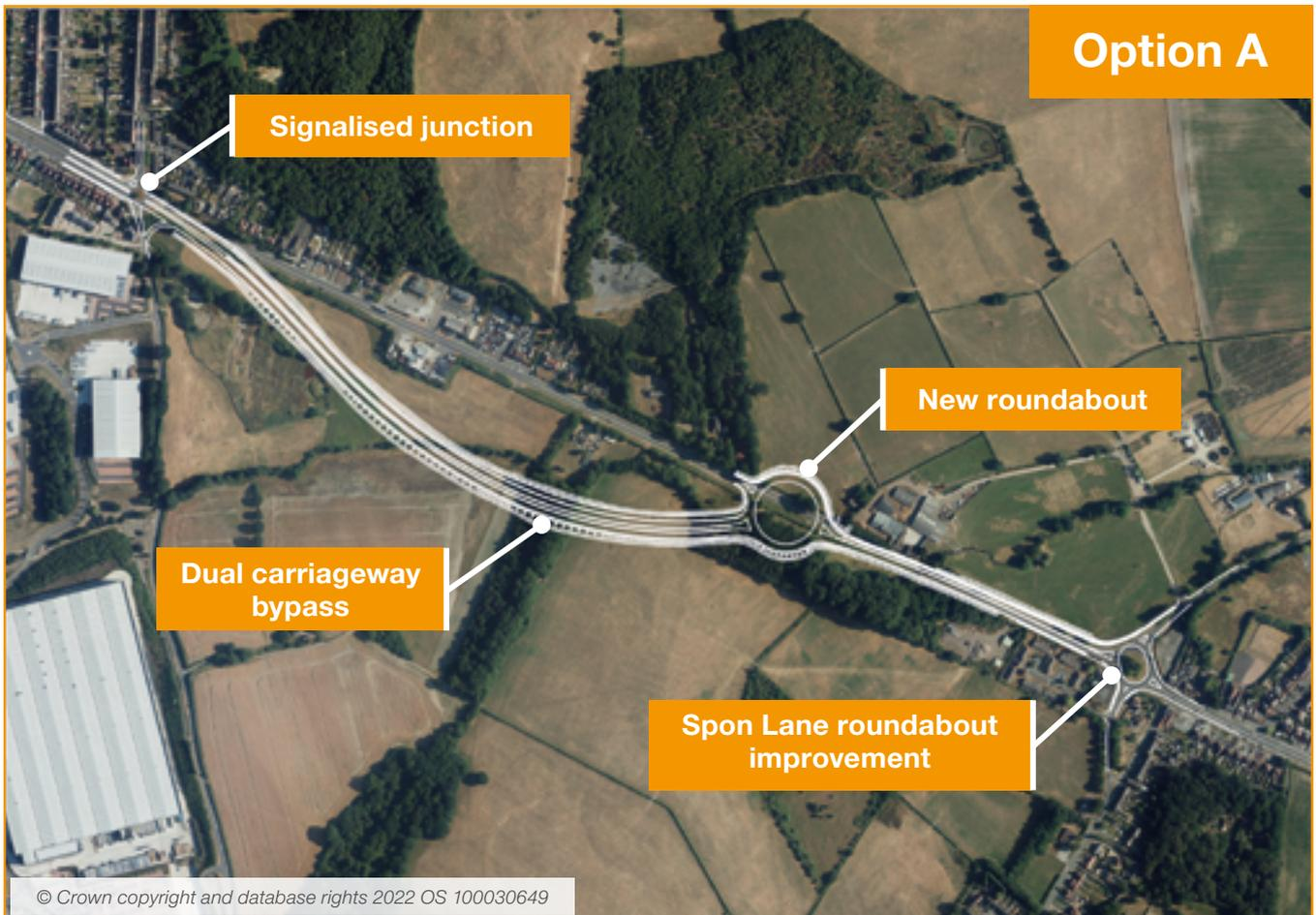
Option A introduces a dual carriageway bypass to the south of the existing A5 corridor and ties into the A5 at the Dordon roundabout. The Dordon roundabout will be upgraded to a four-way signalised junction, maintaining access to Long Street and Gypsy Lane direct from the A5 mainline. A new roundabout is proposed at the eastern end of the bypass to tie back into the existing A5. The existing bypassed section of the A5 is proposed to be de-trunked and will be accessed via the new roundabout.
