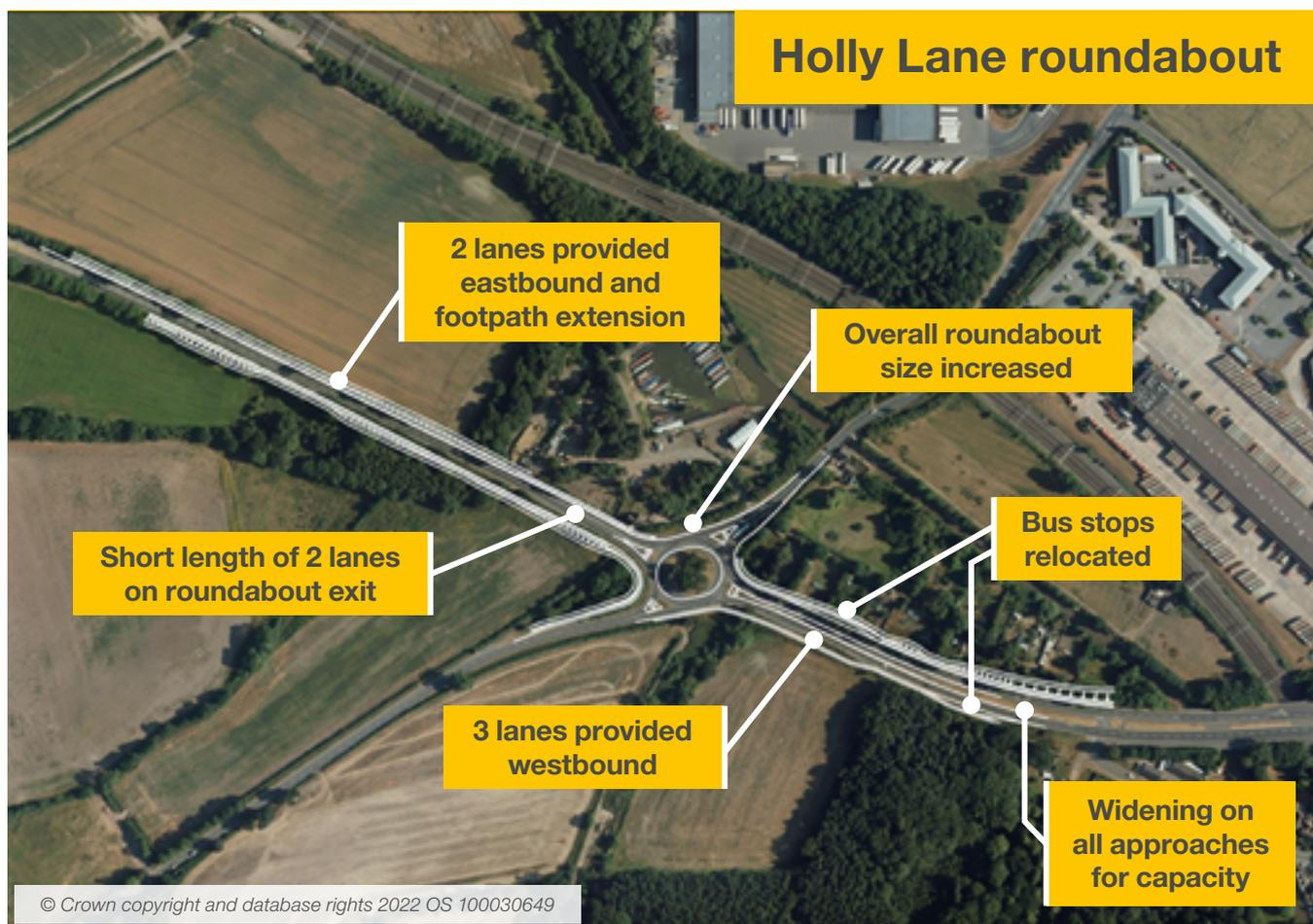
Improvements to Holly Lane will increase the size of the roundabout to provide additional capacity together with footpath and bus stop provision.
