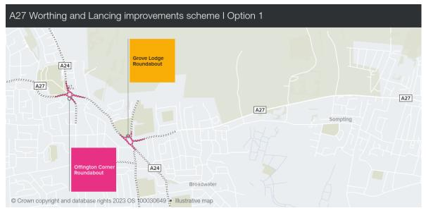
Improvements at Offington Corner Roundabout include widening the roundabout circulatory and several approaches and exits to accommodate additional lanes, which will increase the capacity of the junction and improve the flow of traffic during busy periods. We are also proposing to introduce new traffic lights to the junction to help control vehicle flows and facilitate the safe movement of pedestrians around
