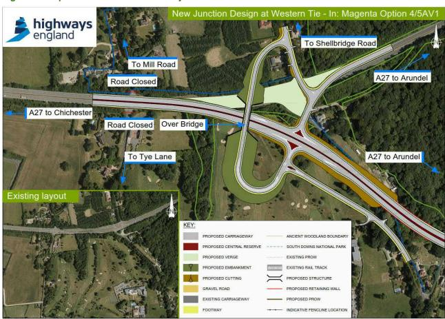
1.4.3 For Option 4/5AV1, a new compact grade separated junction would be provided connecting a realigned Yapton Lane, Shellbridge Road and the existing A27 to the proposed A27. This would allow for all movements onto and off the proposed A27.
