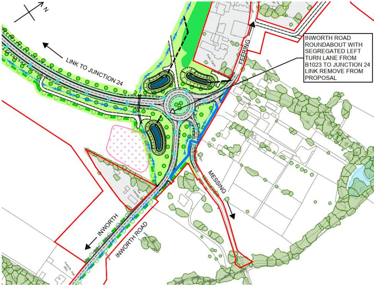
Plate 1.2 Inworth Road Roundabout with Segregated Left Turn Lane removed
