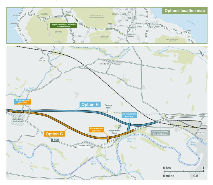
There is a single carriageway for two-and-a-half miles on this section which runs alongside the village of Crackenthorpe. The carriageway varies in width with narrow verges and poor alignment which present visibility issues, particularly at junctions. Local roads junctions and private access points along the route create areas where accidents could potentially occur.
