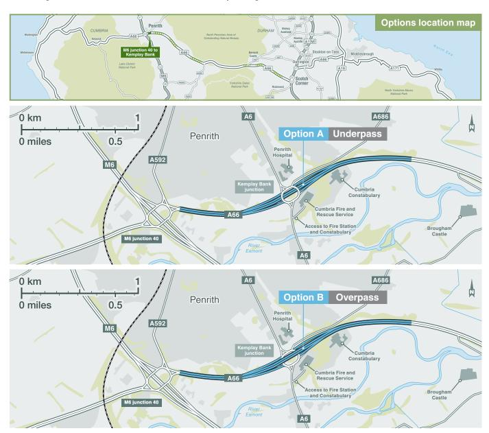
The roundabout can suffer from high levels of congestion which impacts on the flow of traffic along the A66 and for north and southbound traffic using the A6. This bottleneck can also impact M6 junction 40.
