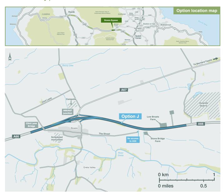
This is a 1.9-mile, single carriageway section which is sandwiched between a dual carriageway to the east and west. A key feature of this section is the junction with the A67 which is currently only accessible to traffic to and from the west.
